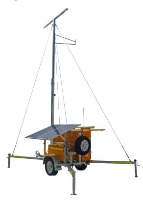
The standard supplied communication boxes are as standard painted in high impact, high visibility yellow and chassis is hot dipped galvanised. Through partnership with leading Queensland painting facilities, the trailer system can be painted to your specific requirement including to MIL-STD and NATO/STANAG standards, such as Olive Drab, Desert Tan, and NATO Green colour schemes.
