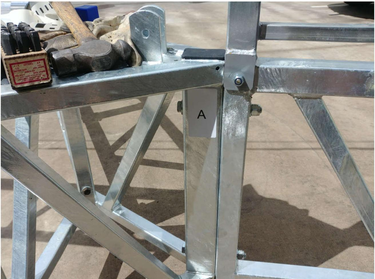
**Step 4. Attach AL340 base module to tripod base.**
