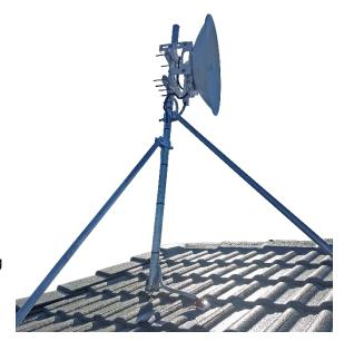
GC48T is a subseries of the traditional GC48 mast, which employs the use of three adjustable threaded bar mounts that fix to the underlying roof structure, such as attaching to rafters or purlins. Installation is a matter of marking out your distances, positioning the plates, and drilling three holes in the tiles to feed the threaded bar through. An M10 bolt runs through a stirrup to hold the central 48 mm diameter pole in place while still pivoting, allowing roof pitch compensation.
